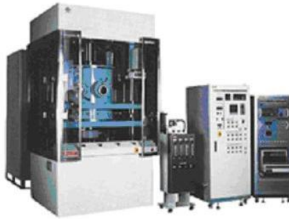
Figure 1 The SPS 7.40 MK-V sintering machine
